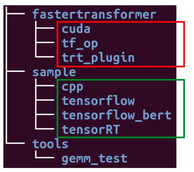
CUDA C++ Implementation, Tensorflow and TensorRT interfaces Sample illustrating how to use it in C++, Tensorflow, and TensorRT
